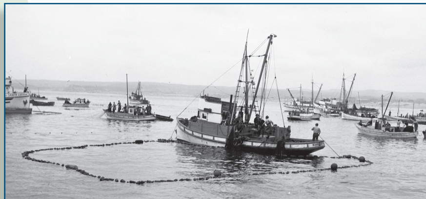
Purse seiner spreading a net for squid, 1957. (J. B. Phillips photograph; courtesy Tim Thomas, Monterey Maritime and History Museum.)
