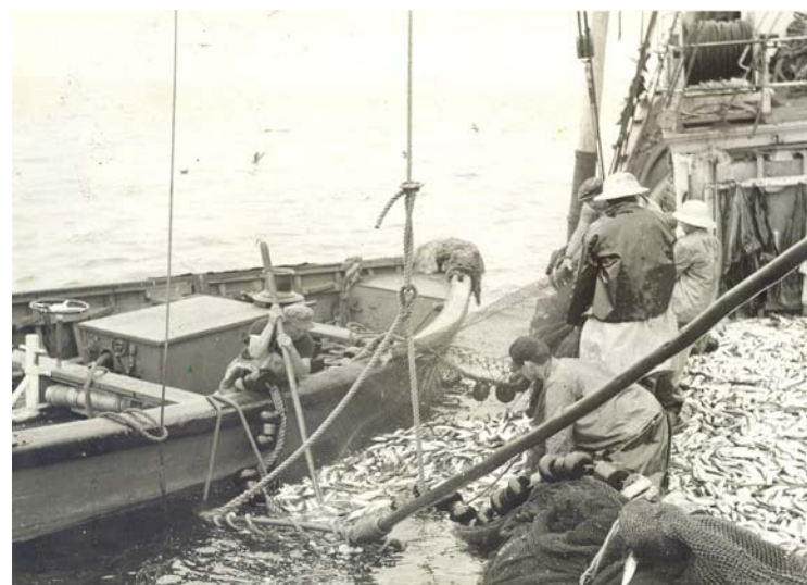
Using a brail net to bring fish on the boat. Courtesy Monterey Maritime and History Museum.
