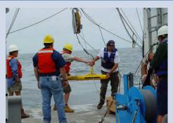
Side Scan Sonar Towfish Being Deployed off a Research Vessel (NOAA/SBNMS)
