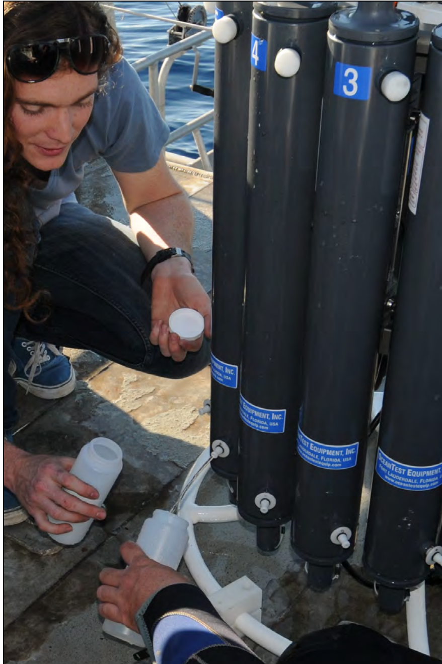
Water samples are collected for nutrient analyses from the sampling carousel aboard the R/V Manta . Photo: NOAA
