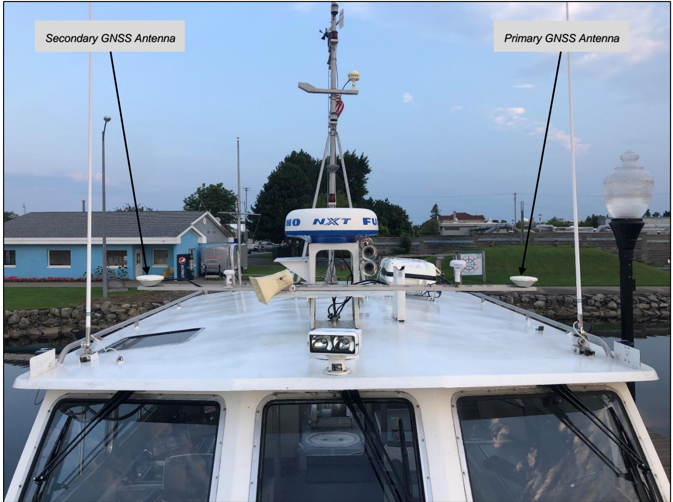
Figure 9. View of POS MV's GNSS antennas installed on R5002 from bow looking aft.
