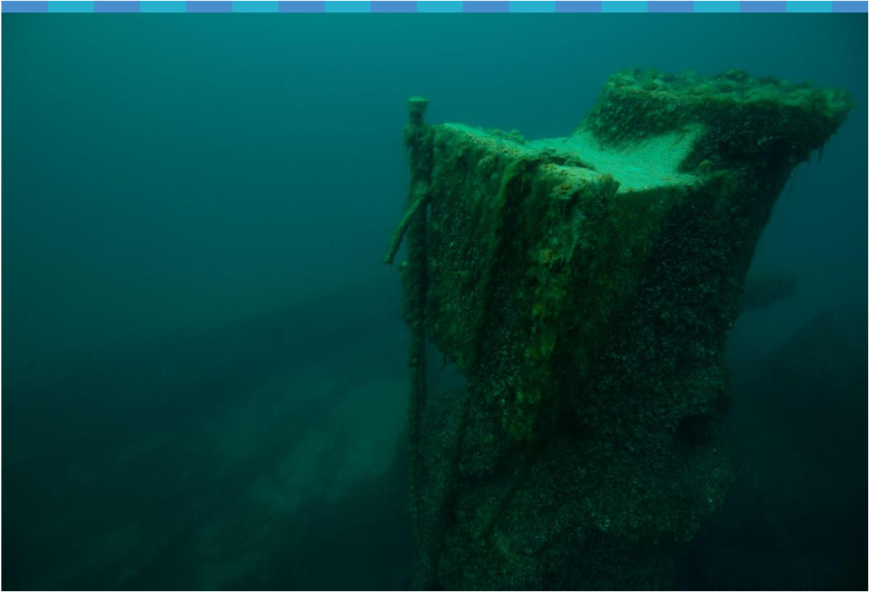
Figure 18. Braided line and chain tied to the engine of Selah Chamberlain ; these lines were formerly used as part of a mooring buoy system but have since been abandoned. Image by NOAA.
