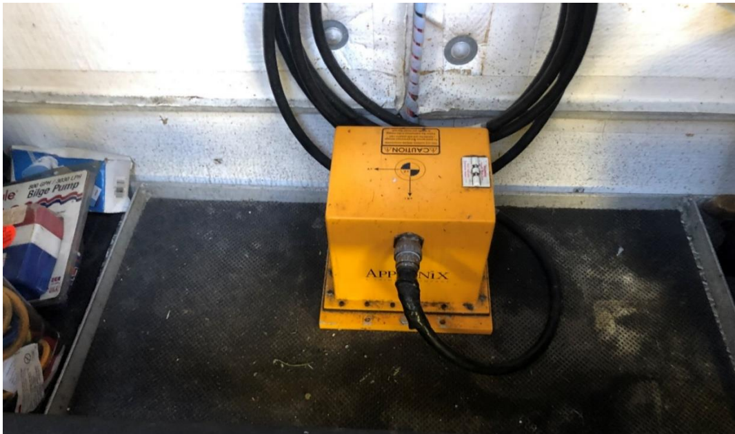
Figure 4. R5002's common reference point for sensor offsets is established at the marked phase center of the inertial navigation system motion reference unit component as shown by the marker on the top of the device.
