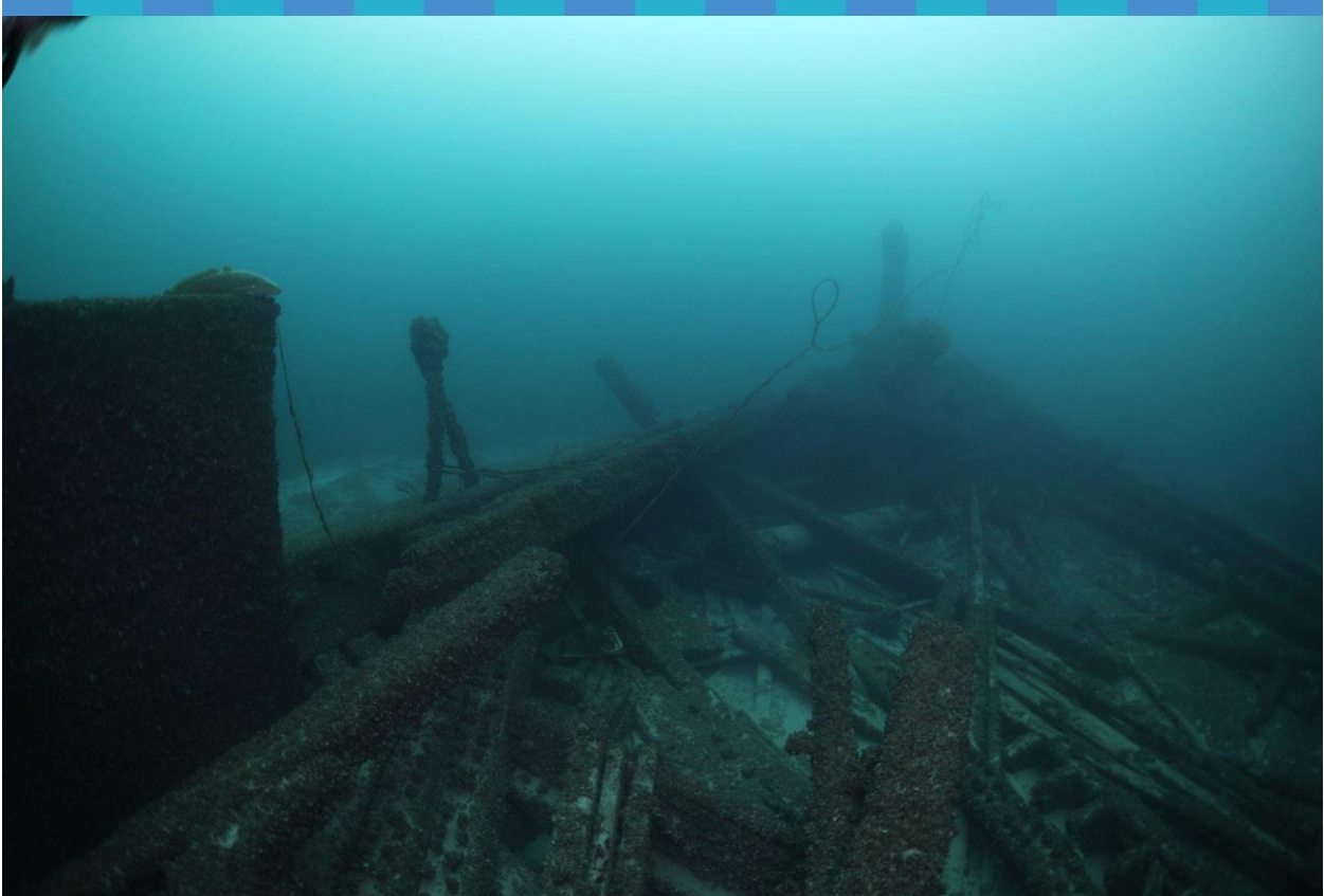
Figure 17. Bow area of America showing fouled polypropylene rope formerly used as mooring lines tied into the shipwreck. Image by NOAA.
