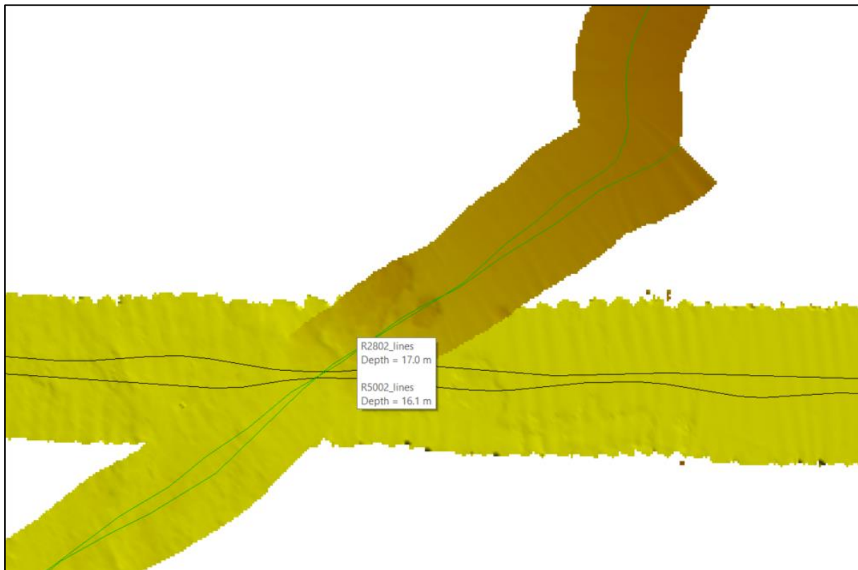
Figure 7. Comparison of calibration data from R2802 and R5002 showing a 0.9 m discrepancy between the datasets despite both being referenced to IGLD85 LWD.
