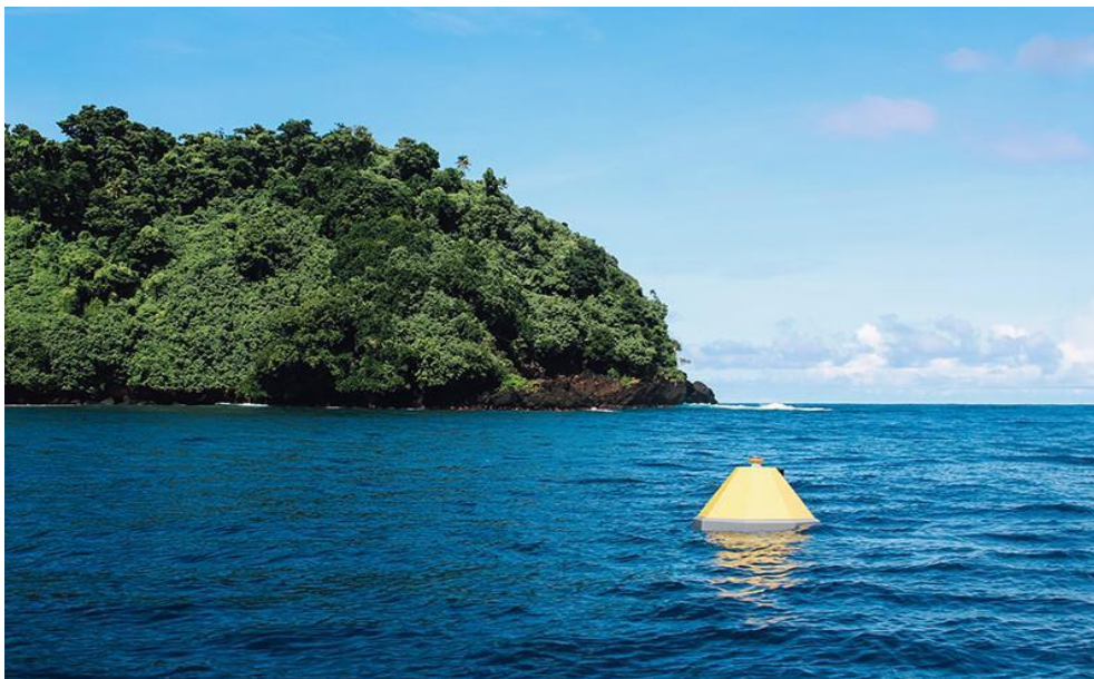
The monitoring buoy in Fagatele Bay collects data on carbon dioxide from surface seawater and the atmosphere as well as data on water temperature, salinity, pH, oxygen, and chlorophyll. Photo: NOAA
