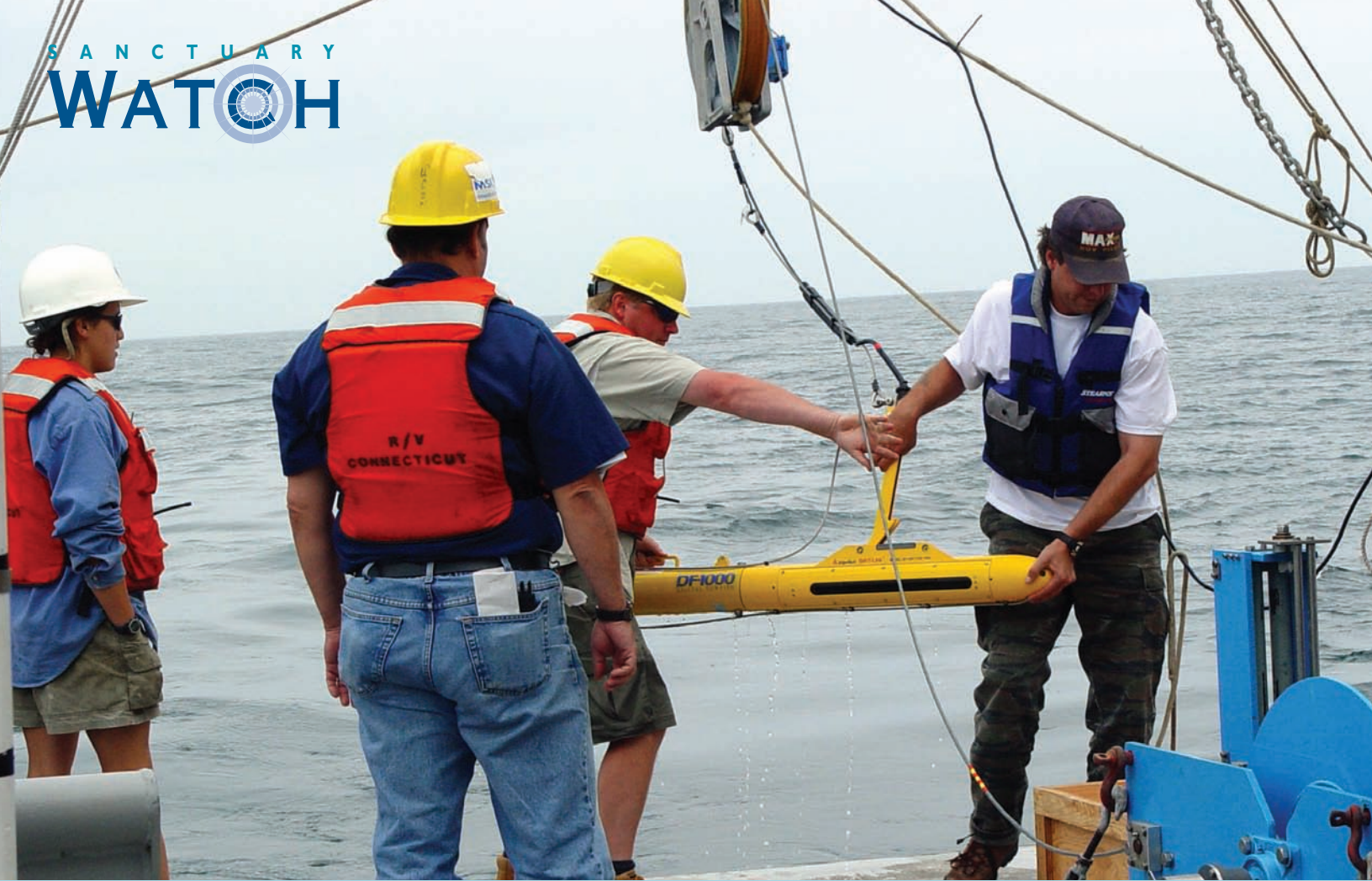
Researchers used a high-tech sonar device like this one to capture detailed images of the wreck of the 19th-century steamer Portland , which rests within Stellwagen Bank National Marine Sanctuary. Photo: Anne Smrcina/SBNMS
