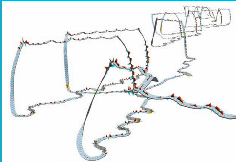
Special software developed at the University of New Hampshire translates data recorded by the D-Tag into an image showing the whale’s movements. Image: SBNMS/UNH
