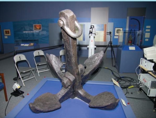
Before: The Monitor 's anchor, on display in the "Ironclad Evidence" gallery at The Mariners' Museum, is prepared for laser scanning. Photo: The Mariners' Museum
