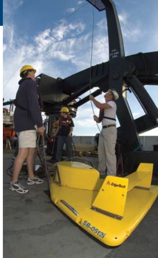
Paul Gayes and a member of the crew clear cables prior to deploying a sub bottom profiler that details rock formations.
