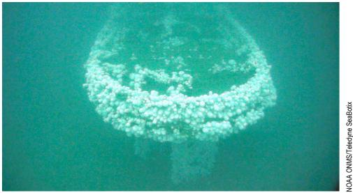
Fig. 15: The stern of the wreck, showing the heavy marine growth and the position of the rudder hard to starboard and steering quadrant on deck hard to port
