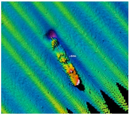
Fig. 3: Multibeam image of Southeast Farallon Island target from Survey H11965 with additional processing and measurement estimates by Gary Fabian.
