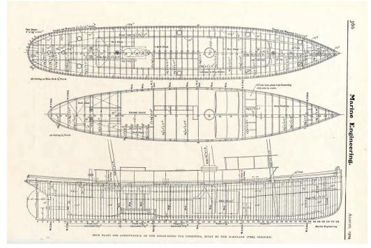
Fig. 18: Deck and Longitudinal View of Conestoga, as reproduced in Marine Engineering (1904)
