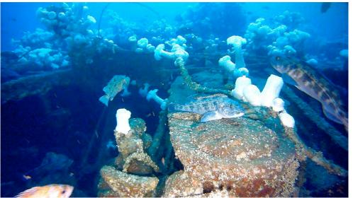
Fig. 10: The engineering spaces lie below the triple-expansion marine steam engine, as shown here in this view looking towards the stern. Loose debris from the superstructure and deck cover the top of the engine's low compression cylinder.
