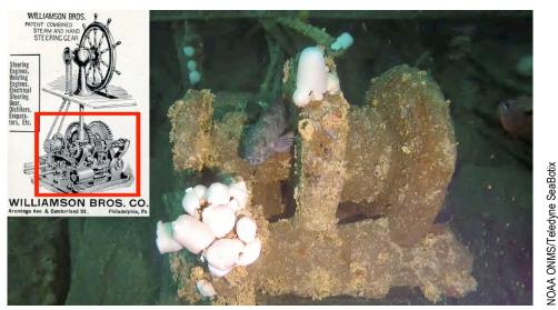
Fig. 7: Williamson Brothers patent combined steam and hand steering gear, lying inside the forward hull next to the 3-inch/50 caliber gun.
