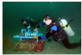
NOAA divers install the seafloor observatory that collects continuous pCO2, pH, and temperature data. Photo Credit NOAA
