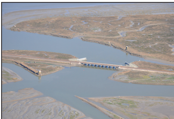
Figure 6. Aerial photo of a sill that was installed at the mouth of Parson’s Slough in 2011. The purpose of this restoration project was to reduce erosion and wetland loss in Elkhorn Slough.
