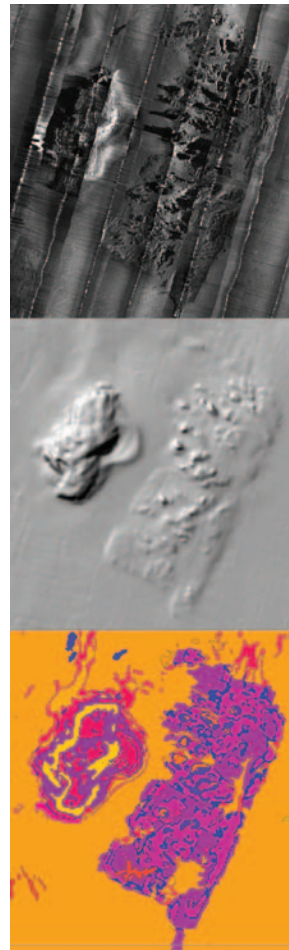
Figure 32. Using texture analysis algorithms, information from side-scan sonar imagery (top plate) and multi-beam bathymetry (middle plate) are combined to create classified habitat images (bottom plate). Image: OCNMS
