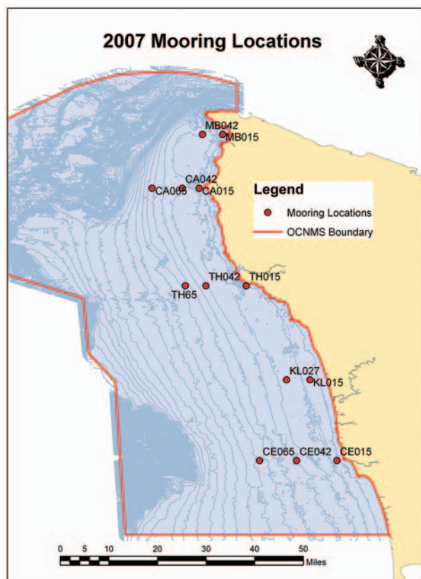
Figure 30. Remote sensors on fixed moorings collect information on physical and biological properties of sanctuary waters at 13 locations that were selected to capture variability in nearshore ocean processes. Source: OCNMS
