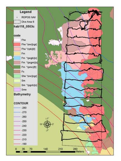
Figure 3. Survey site 6, illustrating the manually delineated polygon as drawn around mosaicked side scan sonar data, the ROV navigation track for the transects surveyed, and the segmented habitat classification polygons according to Greene et al. (1999). See below for key to codes.
