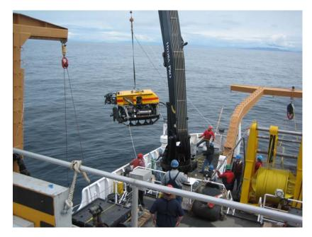
Figure 6. Launch/recovery of the ROPOS ROV off the NOAA Ship McArthur II.
