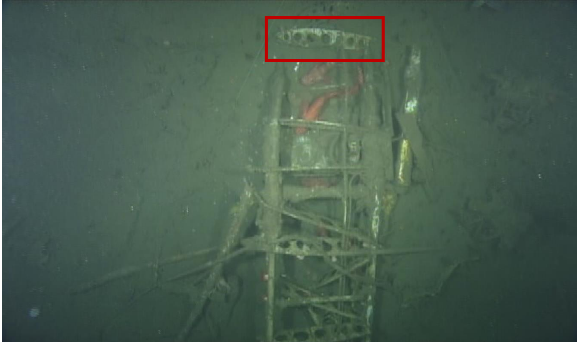
Figure 11- Starboard wing of biplane 3, outlined box shows disarticulated rib. (MBARI, NOAA)
